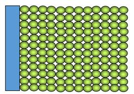
Consider a *one micron* (10 <sup>-6</sup>m) layer of particles with a diameter of 20 nm and a porosity of 50% spread on a 1 cm<sup>2</sup> flat electrode
