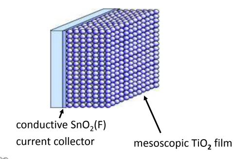
Advantage of nanocrystalline Oxides electrodes:
