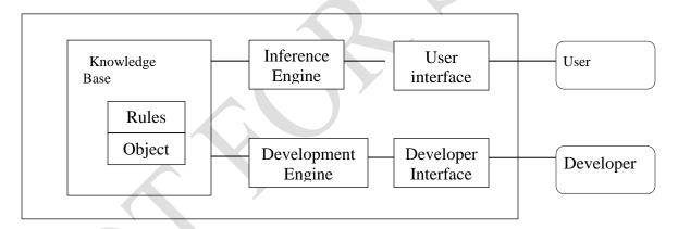
(b) An expert system consists of several components. The above figure illustrates components of an expert from both user and developer perspectives.
